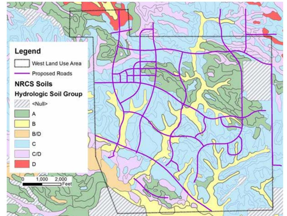
Figure 101: Soils map of the project area indicating general suitability of soils for infiltration-based stormwater BMPs (A = good infiltration potential, D = poor infiltration potential). See the area specific soils map in the Appendix for more information.
