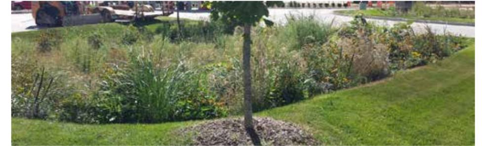
Figure 115: Example of on-site detention, in this case a pair of small basins on a gas station site, planted with native vegetation.
