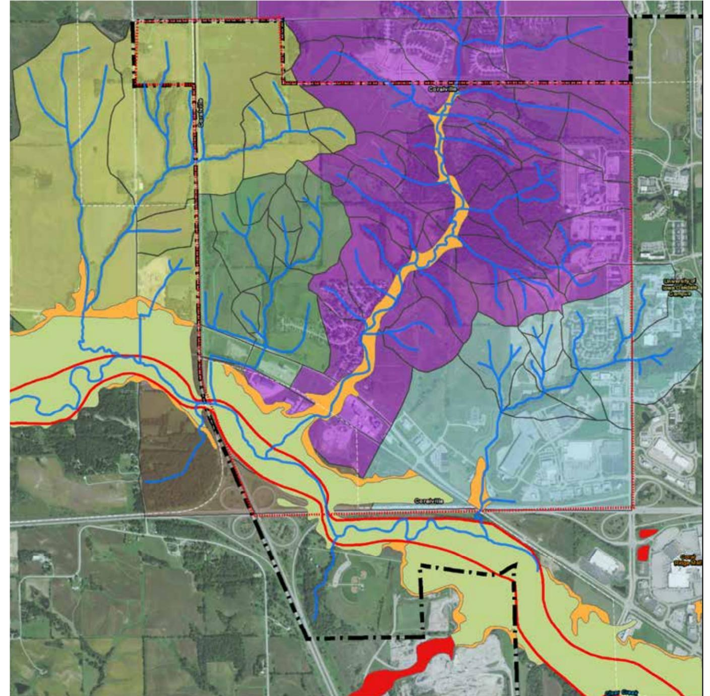
Figure 100: The West Land Use Area showing delineated watersheds, drainage basins, stream lines, and regulatory floodplains
