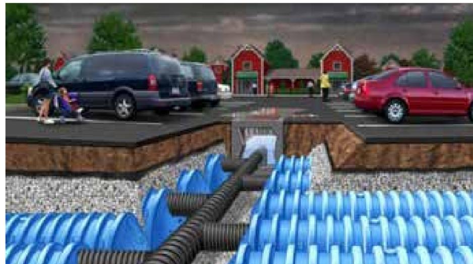
Figure 117: Example of an underground detention system (image courtesy of hydrocad.net)
